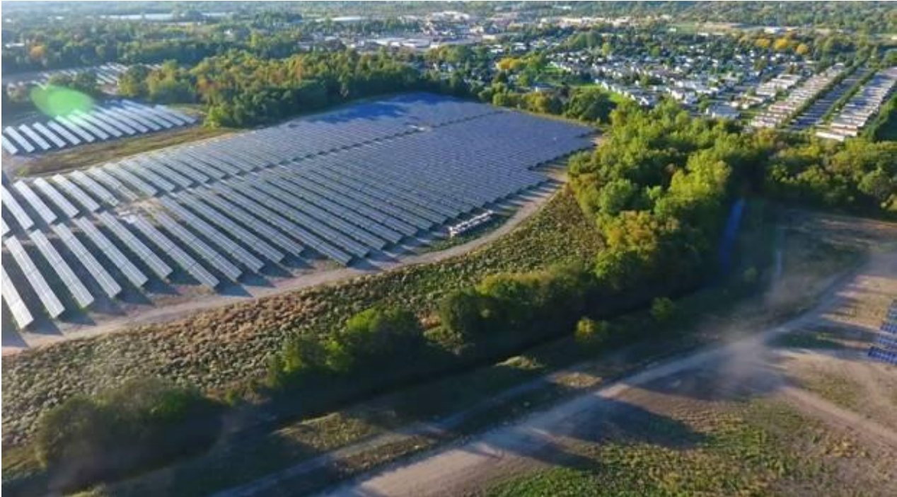
Example of single axis tracking aerial layout. Note north/south configuration (this is not an actual project; just a random piece of land)
